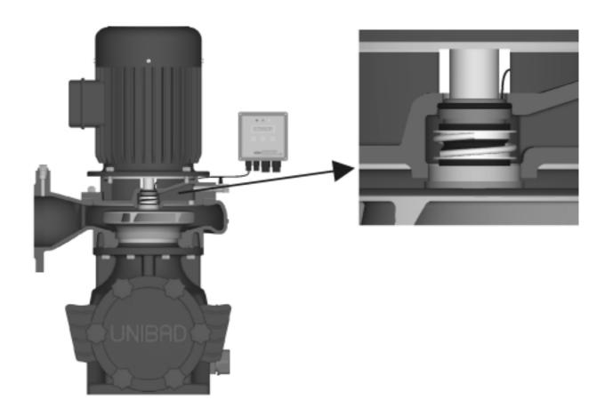
Figure 1 Position of the sensor
