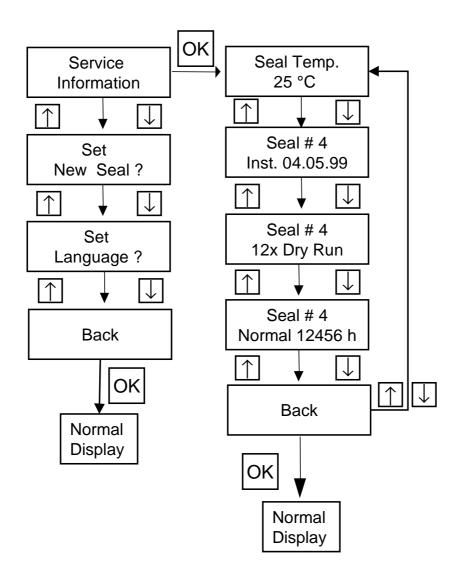
From the normal display, you get to the menu item "Service Information" by pressing  $[\Psi]$ . Pressing [OK] will display the current seal temperature. By repeatedly pressing  $[\Psi]$  or  $[\Lambda]$  you can navigate through the following menu items:
